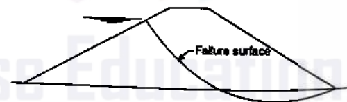
FIG. 10.7. DEEP D/S SLIDES DURING STEADY SEEPAGE.
