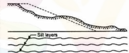
FIG. 10.8. FAILURE BY SPREADING
