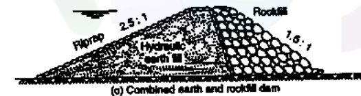
FIG. 7.9 EARTH AND ROCKFILL DAMS.
