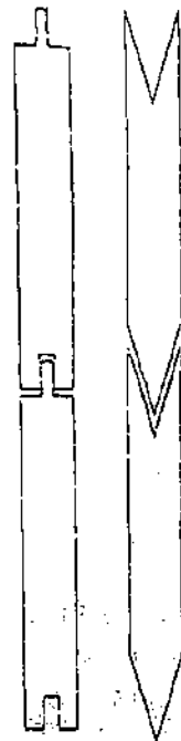
(a) Tongued and grooved joint (b) V-joint
