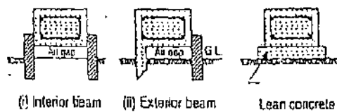
(c) Beam in expansive soils (c) Beam in non-expansive soil
